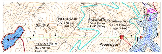
Fig 6. General Layout of Mirabad pumped Storage site
