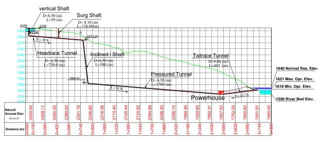
Fig 7. Longitudinal Section of Mirabad pumped Storage Hydro Power
